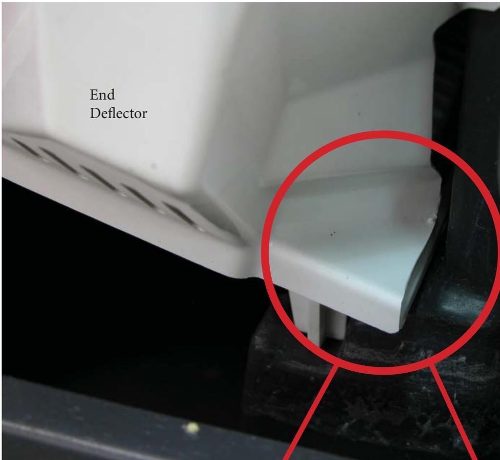
The End Deflector must be in place as shown here. The End Deflector routes the ice towards the cube chute outlet AND holds the cube deflector so it does not move.
